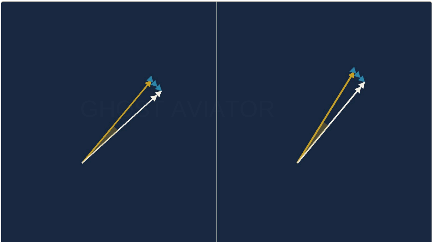
Figure 8.7 — A heading change that leaves the drift where it was. The two wedges are the same size. This is the comfortable case, and it is the one the last example happened to be.
