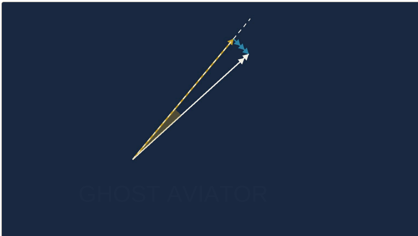
Figure 8.4 — Heading 040° gives a track of 048°. The wedge between the white ground vector and the track you wanted is the whole problem, and over 100 nautical miles it is fourteen miles of error.
