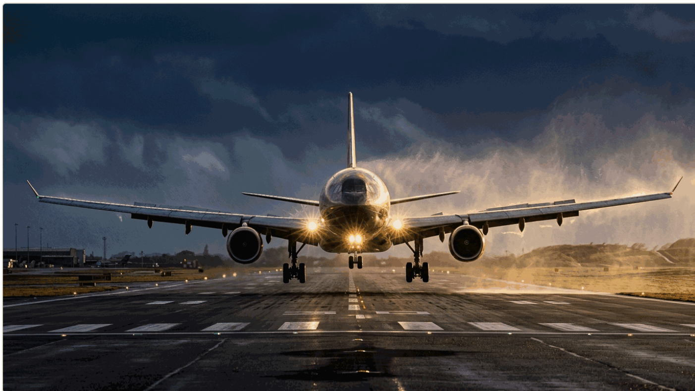
Figure 7.11 — Short final, strong crosswind. The nose is pointing well off the centreline and the aeroplane is tracking straight down it. Nothing is wrong. This is what competence looks like.
