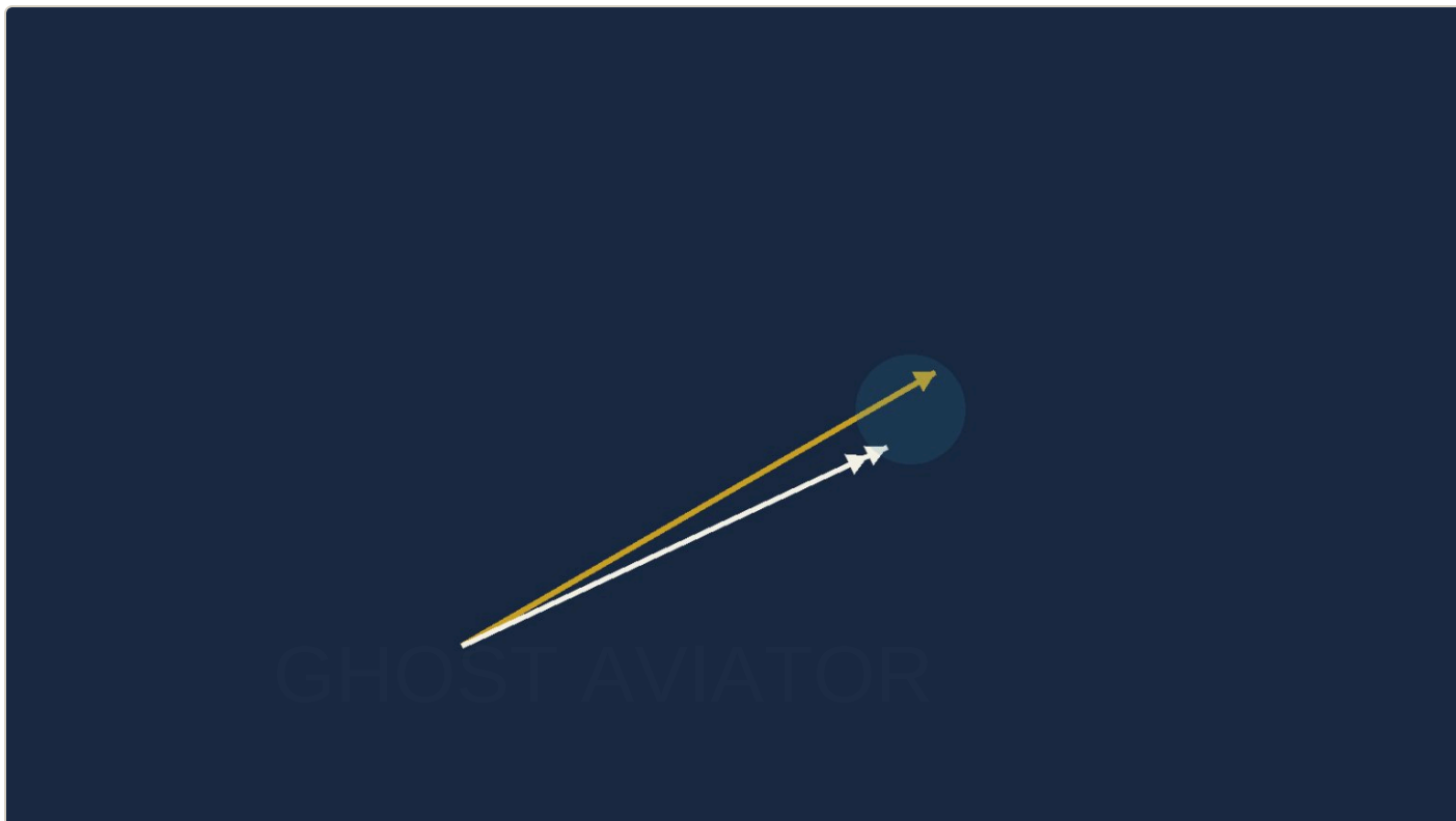
Figure 8.14 — Two sides of the triangle, measured rather than forecast. The gap between the two arrowheads is the wind, and it has been there all along.
