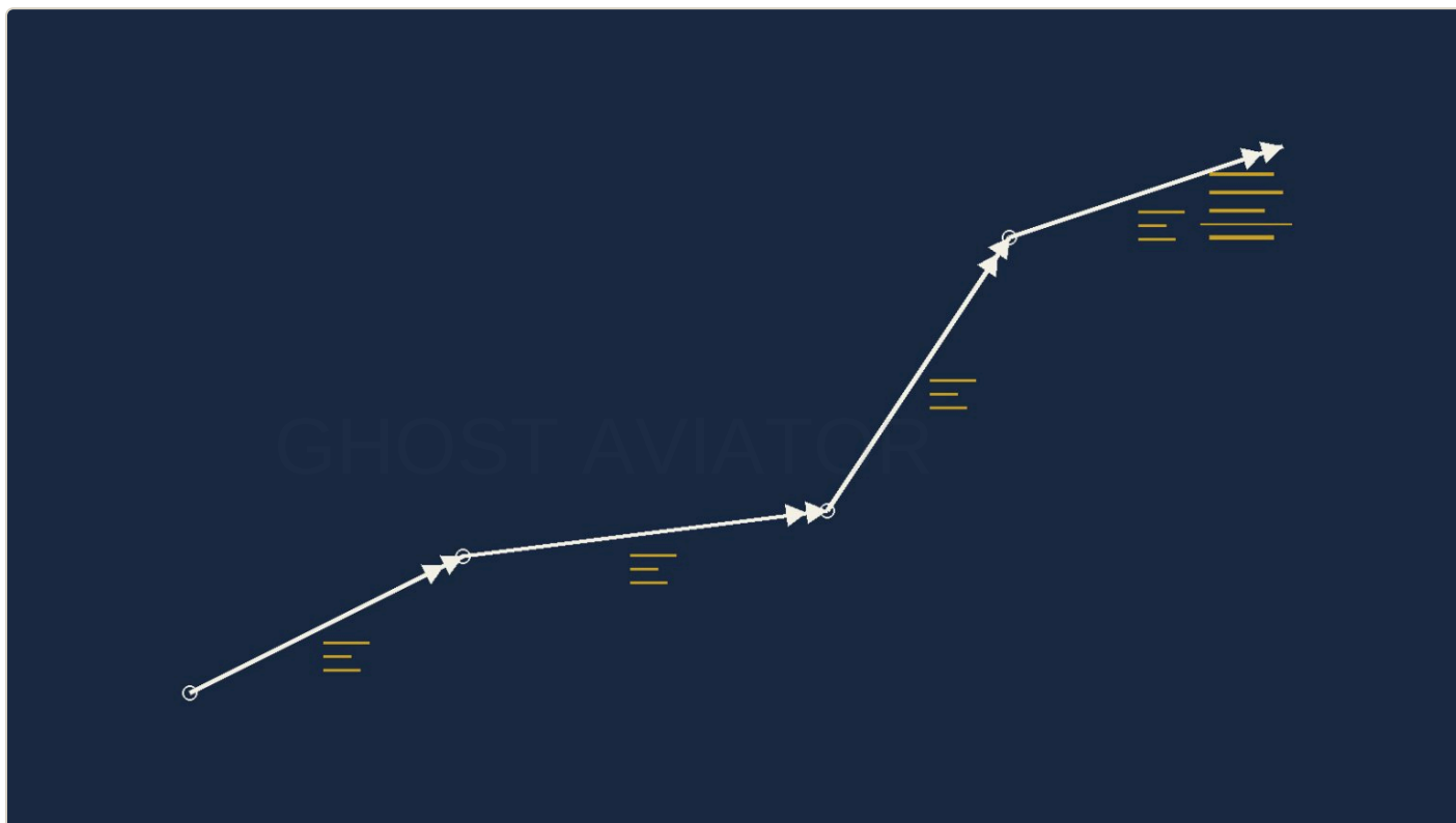
Figure 8.12 — A trip is legs, and legs share almost everything. The aircraft does not change TAS between turning points; the variation barely moves; the fuel flow is a property of the engine, not of the leg. The machine knows this.
