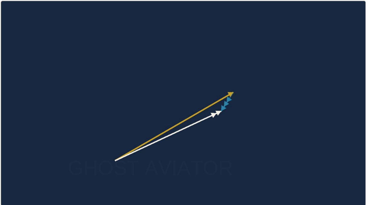
Figure 8.15 — The triangle closes, and the closing side is the answer. Note where it starts and where it ends: from the air vector's tip, to the ground vector's tip . Draw it the other way round and you have the reciprocal, which is the single commonest error in this operation.
