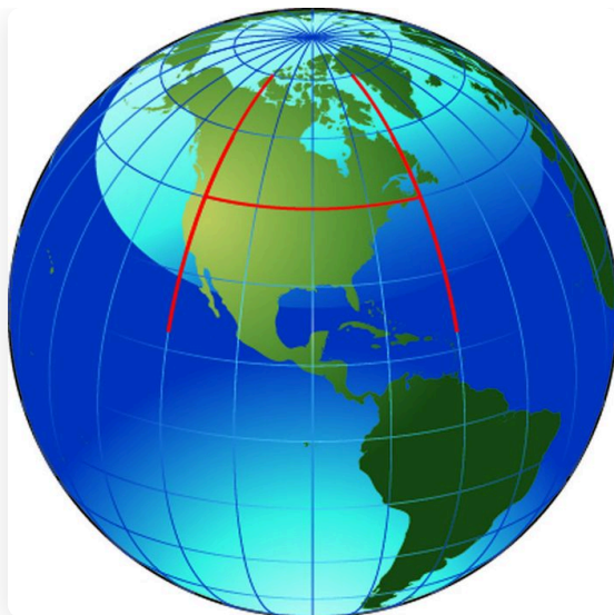
Figure 5 — Two meridians joined by a parallel of latitude — the east-west measurement is departure
