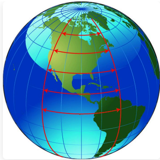
Figure 2 — Effect of latitude: the same ch.long gives shorter departure as latitude increases toward the poles
